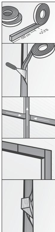
**Preparation of joint/application base:** The application area/ pressure base should be as level as possible and cleaned (eg plaster leftovers removed completely). The joints should run parallel where possible (in some cases a re-plastering or re-profiling of the joints in older buildings could be necessary). The specified tape widths should not be exceeded or reduced and this also applies to use on uneven surfaces.
