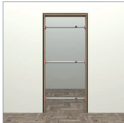
1. Set up the frame and brace it.
