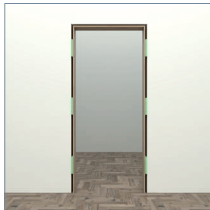
3. After curing, despread and cut off the surplus PU foam.
